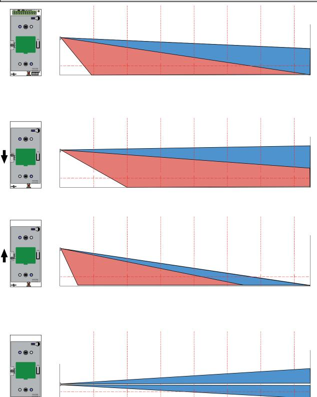
Note: the figures show the effect of the beams based on the position of the board. Since they are purely indicative, we recommend you thoroughly test the sensitivity of the sensor after each adjustment.
