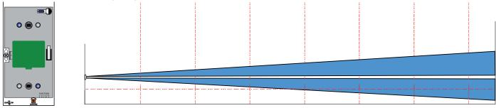
**Using the sensor with 2 vertical curtain lenses:** the use of vertical curtain lenses is based on the need to protect doors and windows with a vertical curtain that is no wider than 50 cm. In this way the protection is only near the doors and/or windows without extending into other areas. You can position the sensor at a height of between 1 m and 2 m based on need. The beam is about 50 cm wide for an aperture of about 90/100 vertical degrees (fig. below)
