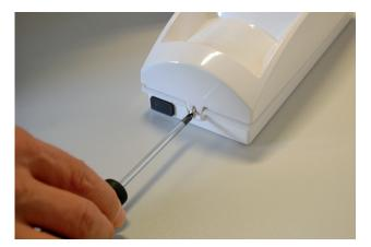
Remove the board, making a hole in the back of the upper cover for the cable to pass through in a suitable installation position. Make another 2 holes to attach the sensor to the wall. We recommend using anchors that are no smaller than 3 mm.
