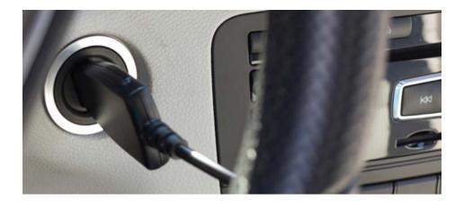
Connect Smart Pro Tester to vehicle via OBD connection.
