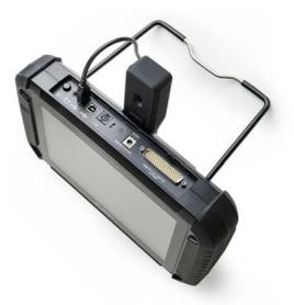
The Smart Programmer connects to the USB Port on the top of the Smart Pro.
